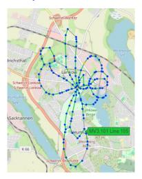
The goal of this thesis is to develop a software prototype that can be used to make graphical changes to this grid model. The grid and its participants, such as loads and photovoltaic systems, nodes and lines, transformers, etc. should be possible to visualise. Furthermore, the user should be able to edit grid data smoothly, e.g. via drag-and-drop, and these changes should be transferred to the PSDM accordingly. The prototype will be validated and tested.
